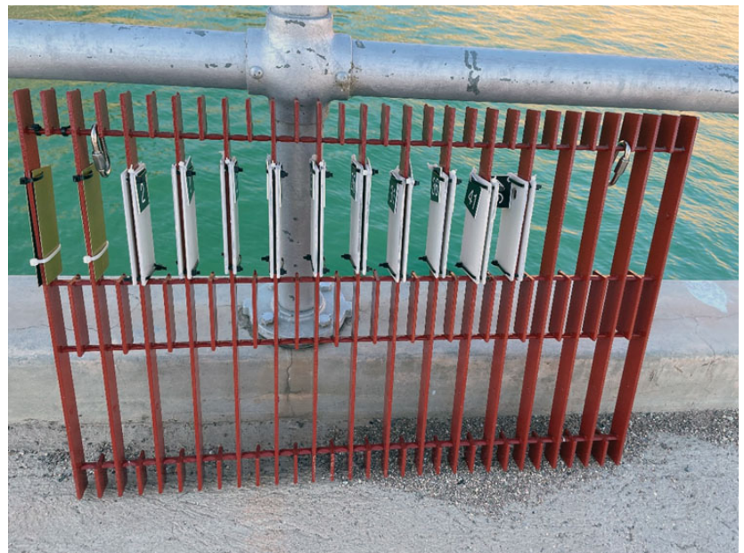
Experimental test rack prior to installation for testing. Pannels are experimental formulations that have been designed to have increased durability and longer service lives.
